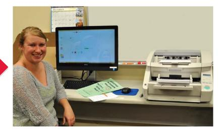
The ImageCast® Central is used to tabulate results from all ballots and all voting channels. As ballots are scanned, the system automatically digitally out-stacks ballot images needing review - our Adjudication application then takes over. The Adjudication application is the digital tool that provides real time efficient multi-user adjudication of ballots, with customer-defined out-stack conditions.
